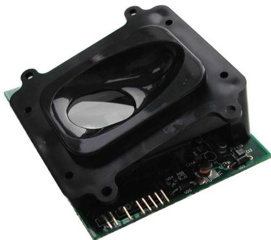
Fingerprint images and templates can be transferred between FS83 and host system for making flexible application. Futronic provides development tools to customer free of charge for integrating the FS83 with host system.
